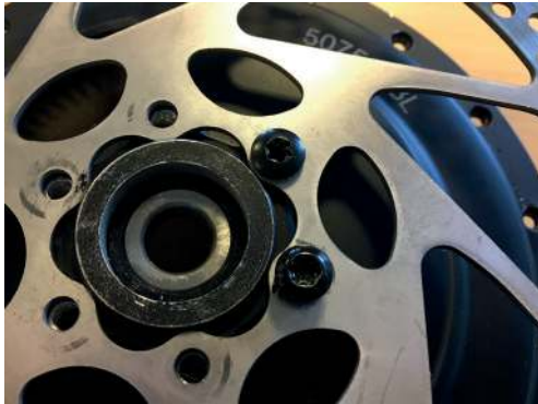
Replacement of disc brake with screws from the motor.
